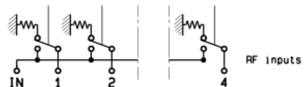
Single Pole n Throw Terminated Switch (n<13) Same as SPnT, but each unused output port is automatically terminated in an internal 50 Ohm resistive load.
